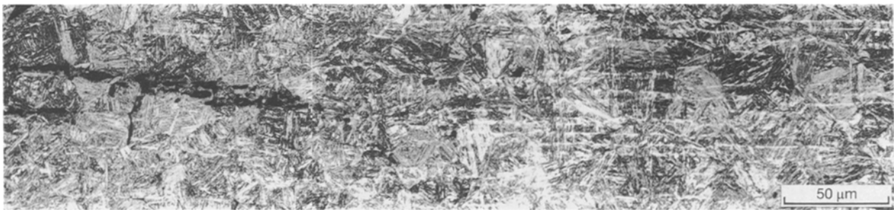
Figure 4 Microstructure of secondary crack beneath the main fracture surface.
